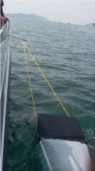
A photograph of a trawl transect site. A yellow rope is attached to a boat, and a black trawl net is being pulled through the water. The background shows a wide expanse of blue water and distant mountains. |
